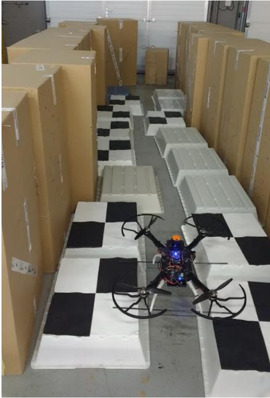
Figure 11: Example setups for lab tests: (left) altitude control tests with simulated uneven ground and walls (right) flight underneath obstacle with 60cm clearance like in Mercat del Born
