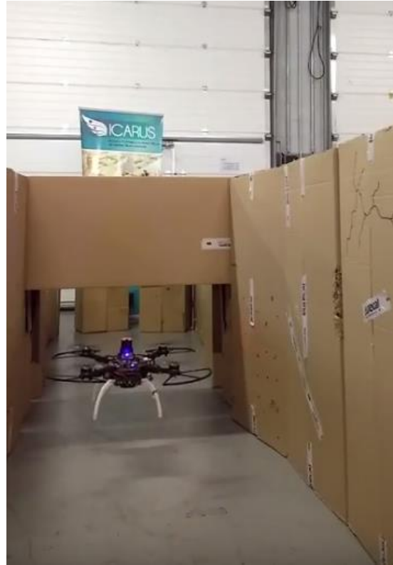
Figure 11: Example setups for lab tests: (left) altitude control tests with simulated uneven ground and walls (right) flight underneath obstacle with 60cm clearance like in Mercat del Born
